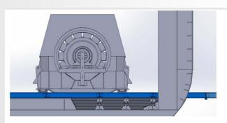
The profile chosen for this beam is W10 x 10 x 112, with an elastic section modulus  $W_Z$ = 2078  $cm^3$
