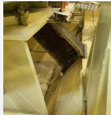
RESONANCE SOLVING: VIBRATIONS LEVELS REDUCED FROM 18MM/S TO 4/MMS COMPARING BEFORE AND AFTER REINFORCEMENT
