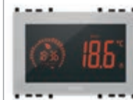
02955.N Touch screen timer-thermostat for ON/OFF and PID temperature control, 1 input for temperature sensor, 1 multi-function input, 1 RJ9 input for energy meter (02960), 5(2) A 230 V~ change-over relay output - 3 modules. Depth: 35,3 mm
