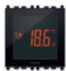
02950 Touch screen thermostat for ON/OFF and PID temperature control, 1 input for temperature sensor, 1 multi-function input, 5(2) A 230 V~ change-over relay output - 2 modules. Depth: 38,5 mm
