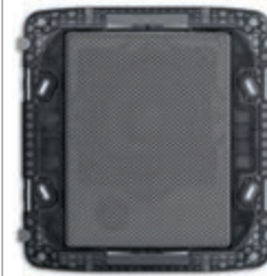
21588.N Passive speaker, 8 Ω 10 W, with built-in 8-module mounting frame. Depth: 48 mm
