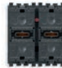
20527.1 2 rocker push buttons + actuator 1 roller shutter laths positioning, cosφ 0,6 2 A 120-230 V~ - 2 modules. Depth: 37 mm
