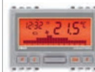
20446.N 5(2) A 250 V~ change-over relay output, AA LR6 1,5 V battery (supplied) - 3 modules. Depth: 43 mm
