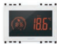
02955.B Touch screen timer-thermostat for ON/OFF and PID temperature control, 1 input for temperature sensor, 1 multi-function input, 1 RJ9 input for energy meter (02960), 5(2) A 230 V~ change-over relay output - 3 modules. Depth: 35,3 mm
