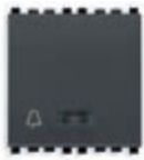
20183 For emergency call, 2 NO 5 A 250 V~, 12 V~/12-24 Vdc (SELV) - 2 modules. Depth: 38,5 mm
