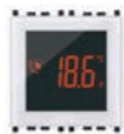
02950.B Touch screen thermostat for ON/OFF and PID temperature control, 1 input for temperature sensor, 1 multi-function input, 5(2) A 230 V~ change-over relay output - 2 modules. Depth: 38,5 mm
