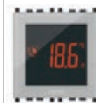
02950.N Touch screen thermostat for ON/OFF and PID temperature control, 1 input for temperature sensor, 1 multi-function input, 5(2) A 230 V~ change-over relay output - 2 modules. Depth: 38,5 mm
