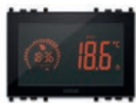
02955 Touch screen timer-thermostat for ON/OFF and PID temperature control, 1 input for temperature sensor, 1 multi-function input, 1 RJ9 input for energy meter (02960), 5(2) A 230 V~ change-over relay output - 3 modules. Depth: 35,3 mm
