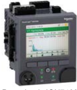
PowerLogic ION7400 with harmonics display.
